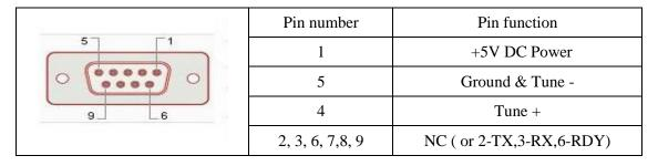
The module is preset to customer needs, can be operated without control software. RS232 communication code and controller software can be provided upon the request.
